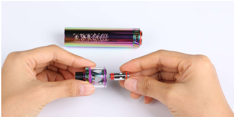
A vaping device deconstructed ... the heating element and the battery power source are shown here.
